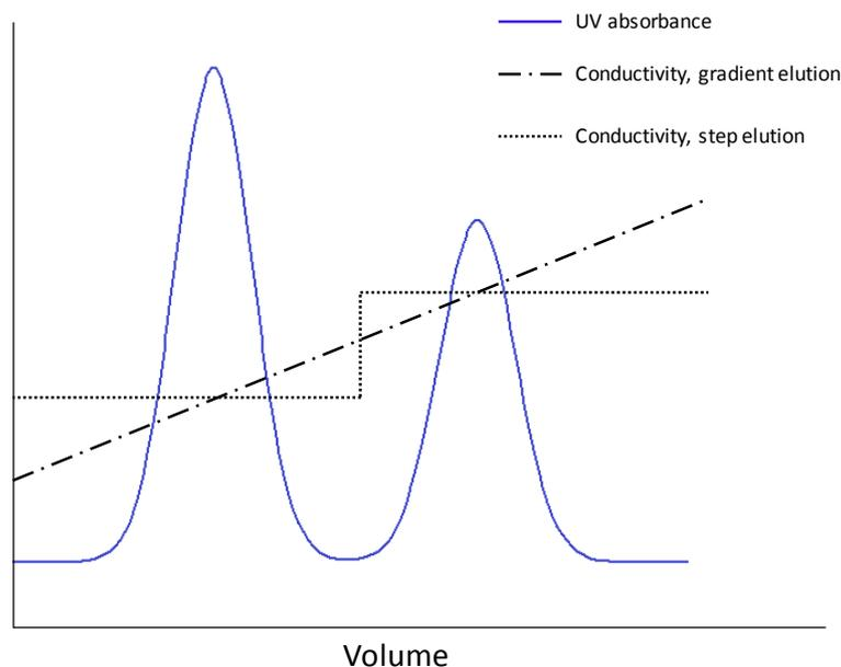
Figure 2. Optimization of step elution with salt. A test run with linear gradient elution gives information about suitable salt concentrations to be used in the step elution. Note: Remember to take the system dead volume into account when comparing the print out of the gradient and the trace.
