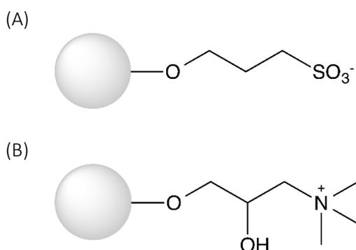
Figure 1. Structure of the ligand used in WorkBeads 40S (A) and WorkBeads 40Q (B).
